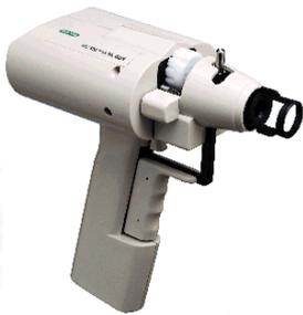
The image shows a Biolistic Particle Delivery System (BPDS) gun, which is used for the direct delivery of DNA-coated particles into plant cells. The background features a faint image of a llama and a plant.
